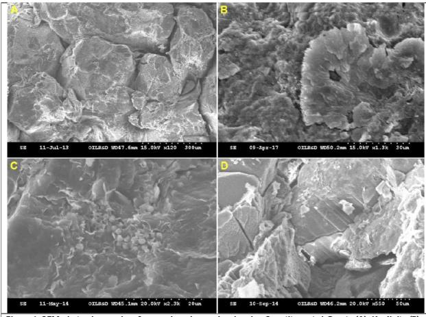
Figure 4: SEM photomicrographs of reservoir rock samples showing Smectite coated Quartz (A), Kaolinite (B), Pyrite-Illite (C) and Feldspar (D).
