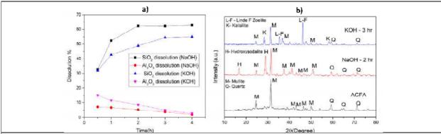
Figure 1. a) Effect of leaching time on the dissolution of Si and Al for NaOH and KOH. b) XRD patterns of ACFA, NaOH treated CFA and KOH treated CFA at optimum leaching time.
