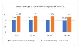
Fig.4.Comparison Graph of Compressive Strength for NC and RAC
