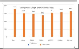
Fig.10.Comparison Graph of Slump Flow Test
