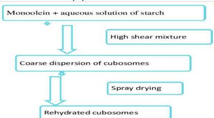
Figure8. Flow chart for the formation of dry powder precursor cubosomes
