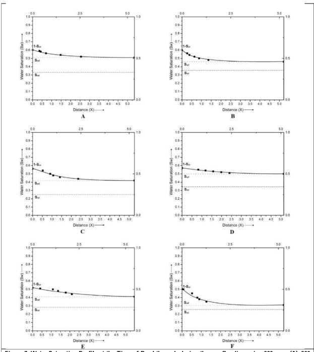
Figure 7: Water Saturation Profile at the Time of Breakthrough during the coreflooding using 200 ppm (A), 500 ppm (B), 800 ppm (C), 1100 ppm (D), 1404 ppm (E) and 2500 ppm (F) brine.
