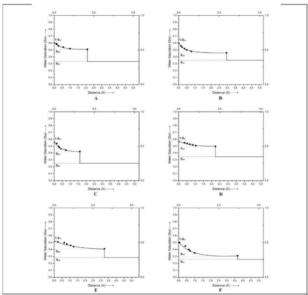
Figure 6: Water Saturation Profile before the Time of Breakthrough during the coreflooding using 200 ppm (A), 500 ppm (B), 800 ppm (C), 1100 ppm (D), 1404 ppm (E) and 2500 ppm (F) brine.
