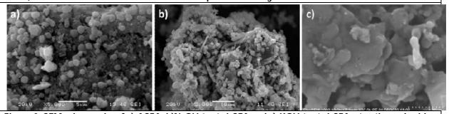
Figure: 2. SEM micrographs of a) ACFA, b)NaOH treated CFA and c) KOH treated CFA, at optimum leaching time.
