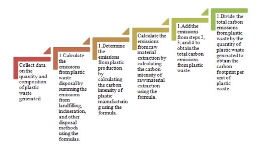
Figure 3 Flow Chart of New Algorithm Calculate the Carbon Footprint of Plastic Waste
