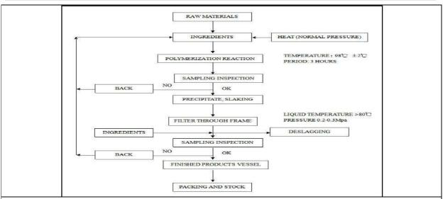
Figure 1.Block diagram of the experimental Process
